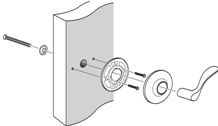
**NOTE:** Carefully follow these instructions when installing. Screws to be tightened to a recommended 2.5Nm torque.
