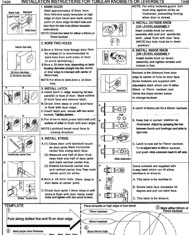
(4) Bore 25.4mm or 24.6mm hole in center of door edge
