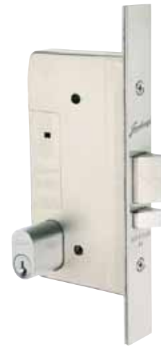
3900 Series Nightlatch (deadlatching) Key or snib retraction of latchbolt No handle/knob furniture
