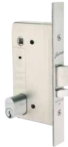
3500 Series Combination lock (deadlatching) Handle/knob locked both sides by key/turnbutton
