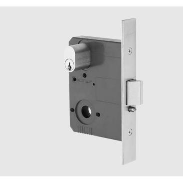
Deadlocking nightlatch featuring a latchbolt which is retracted by a series of cylinders and/or turnbuttons. No handle mechanism.
