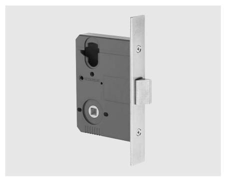
A passage type latch for matching the case dimensions of the range of mortice locks. Features heavy duty springs and same latching as previous latching type locks, but without deadlatching auxiliary bolt.
